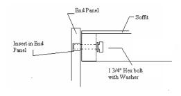
the soffit. Secure with hand tightened 1-3/4" hex bolt and washer through each hole in the soffit into the threaded insert in the end panel. Note 72 and 82h units have inverted soffit.
